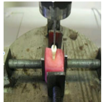
[Table/Fig-4]: Universal testing machine [Table/Fig-5]: Mounted tooth kept on universal testing machine for fracture resistance
